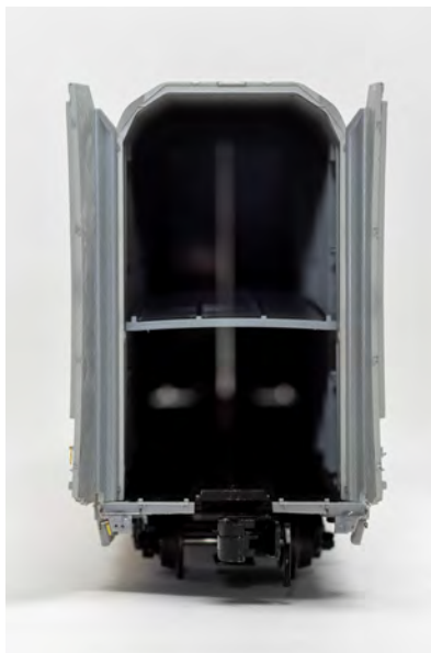
Slide In Interior Deck shown installed
