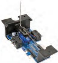
**Horizontal-Mount Switch Machine - Walthers Layout Control System**
