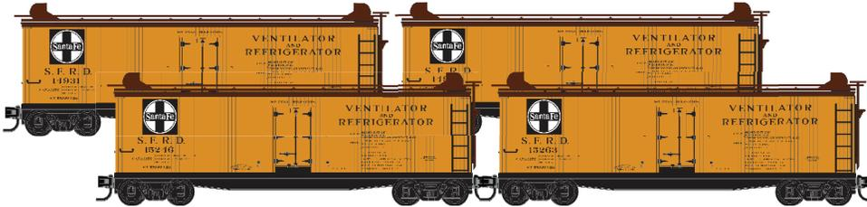
This 40-foot double-sheathed wood ice-reefer, with vertical brake wheel, is black with yellow sides and runs on Andrews trucks. Built in the early-1920s and rebuilt in 1930s, this reefer used 40-ton capacity trucks. This RR-W class car belonged to a series of over 1,250 similar cars, and could be seen in trains all across the country.
