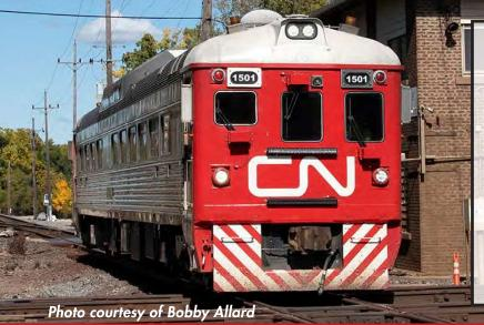
In 2008, Canadian National rebuilt one of their former RDC-1 cars into a Track Geometry Vehicle. Originally built in 1958 as DC-108, it served CN until it was sold to VIA in 1978. Many years later it would be purchased back by CN and undergo an extensive rebuild to analyze their rail network, which consists of over 20,000 rail miles across Canada and the United States. CN 1501 can be seen just about anywhere CN runs and has even been seen on regional railroads!
